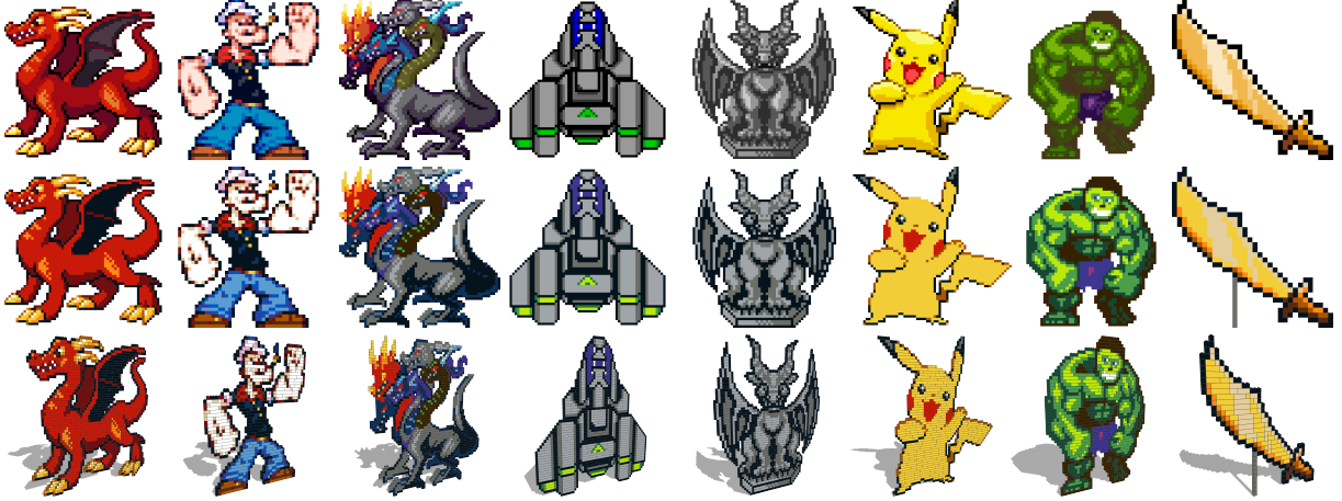
Figure 10: Our framework can generate plausible LEGO brick sculptures from a large variety of pixel art images (see also supplemental material). (Top row) The input pixel art images. (Middle row) The balanced and color remapped 2D shapes. Note that three examples on the right are adjusted to keep balanced by expanding supporting lines (Pikachu and Hulk) or adding supporting strut (Saber). (Bottom row) The final brick sculptures (Input images: “Dragon” and “Hydra” © Heavy Cat Multimedia Ltd., “Popeye” © King Features Syndicate, Inc., “Spaceship” © Asmir Rogo, “Stone Gargoyle” © unrae, “Pikachu” © Pokémon Ltd, “Hulk” © Marvel Worldwide Inc., “Saber” © Manning Leonard Krull).
