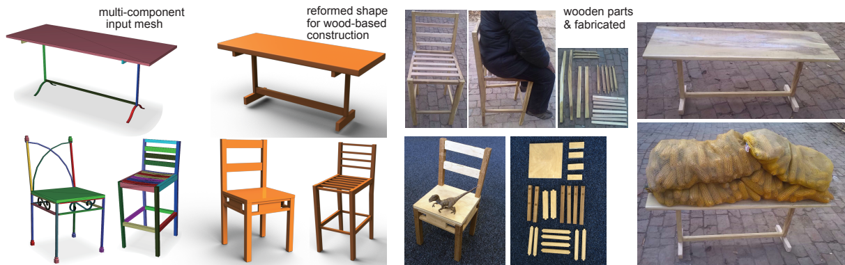
Figure 1: We present a data-driven framework to reform (i.e., reshape) an input multi-component mesh to simplify fabrication from a target built material. The input model (left) can be geometrically and topologically modified to a reformed shape (middle). Part conjoining specifications such as joint information can also be inferred for real fabrication (right).
