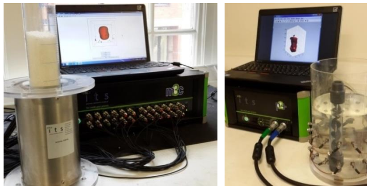
Figure 9: (left) 3x8 ECT and (right) 2x16 ERT experimental setup
