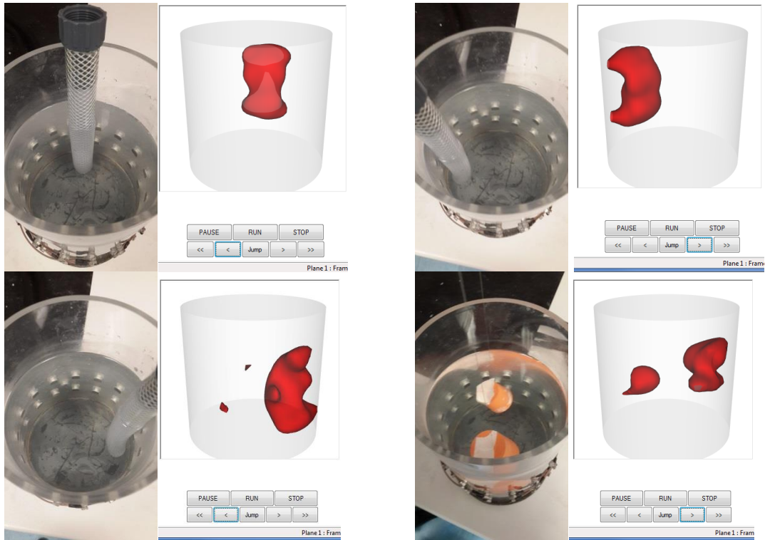
Figure 11: 3D ERT image reconstruction results, showing the locations of non-conductive objects
