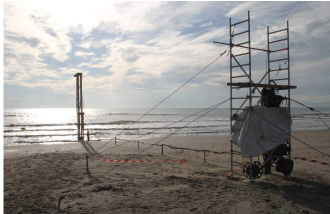
Figure 1: Photograph showing the experimental setup and their location on the upper part of Rousty beach. The TLS was fixed on the 4.8 meters-high tower standing on the left part of the picture while the scaffold is on the right. The buried sensors can be observed in between.
