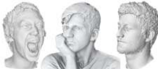
Figure 20.1: Static reconstruction of the head including hair from two images [Blumenthal-Barby and Eisert 14].
