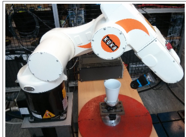
Fig. 1. The new tactile sensor mounted on a KUKA KR5-sixx-R650 robotic arm, currently exploring the tactile appearance of a mug.
