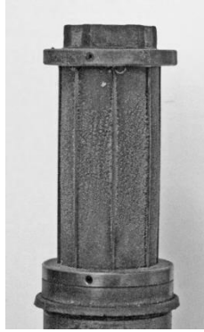
Fig. 16 Photograph of the wired probe after \text{CaSO}_4 fouling test; fluid flows clockwise when viewed from the top
