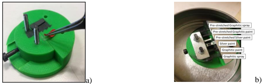
Figure 9 - SEM analysis: a) stretching apparatus; b) samples tested during the analysis
