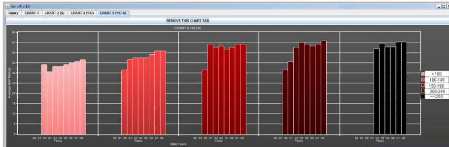
Figure 14: SAP rating chart for loft insulation levels from “i100” to “i=250” mm
