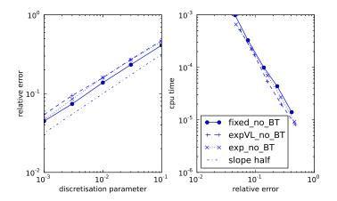
Figure 3: Similar to Figure 1, except the simulations are performed without the boundary tests. Notice that compared to Figure 1, the lines have slope half rather than slope one and the computations are much less accurate (contrast the scale on the error axis).
