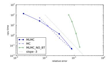
Figure 7: Plots of cpu time against relative error for the computation of the MFET of the FHN example. Three methods are tried, as in Figure 5. The MLMC is applied with  $\Delta t_c = 0.1$  and  $M_k = 100\Delta t_\ell^{-2}\sqrt{\operatorname{Var}(\delta_k)\Delta t_k}$ .
