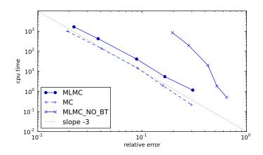
Figure 6: Plots of cpu time against relative error for the computation of the MFET of the OU process with  $\sigma = 0.5$ . The MLMC is applied with  $\Delta t_c = 0.1$  and  $M_k = \Delta t_{\ell}^{-2} \sqrt{\operatorname{Var}(\delta_k) \Delta t_k}$
