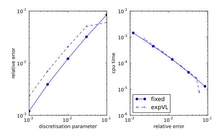
Figure 4: Plots of the relative error against discretisation parameter  $\Delta t = 1/\lambda$  and cpu time against relative error for the FHN model with initial data x = 0 and noise  $\sigma = 0.25$ . The threshold b = 2 and the number of samples  $M = 10^6$ . fixed is the fixed time stepping Euler method with boundary test; expVL is the variant of exp defined by (8). The reference solution T = 2.5677 is used for computation of the relative errors.
