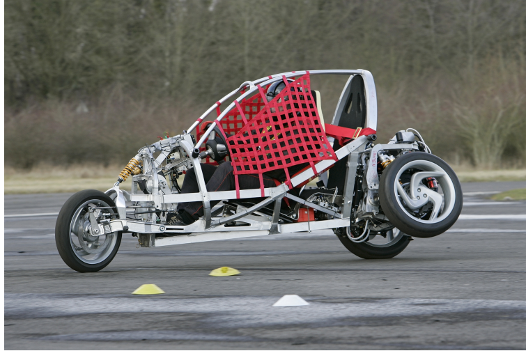
Figure 2: Lifting of inner wheel due to an aggressive steering manoeuvre
