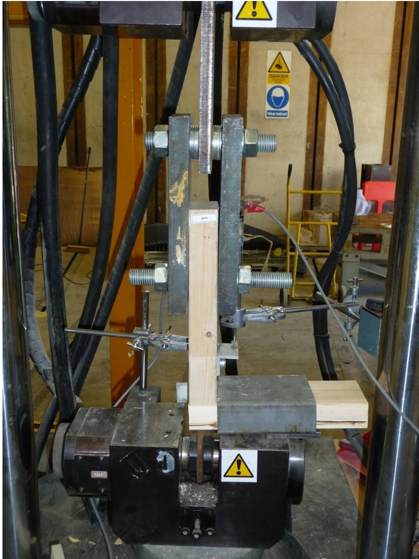
Figure 6 Leading stud joint testing
