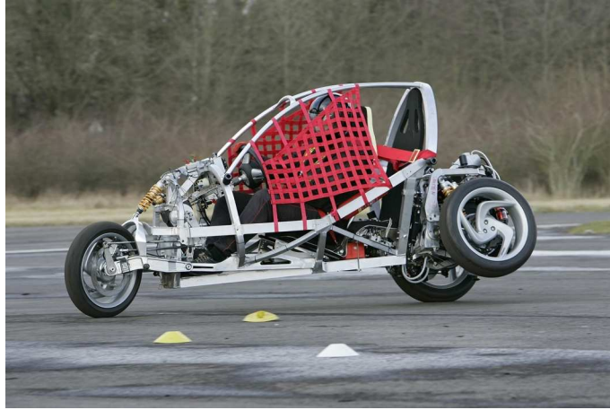
Figure 2: CLEVER Vehicle prototype demonstrating its lack of roll stability in transient conditions.
