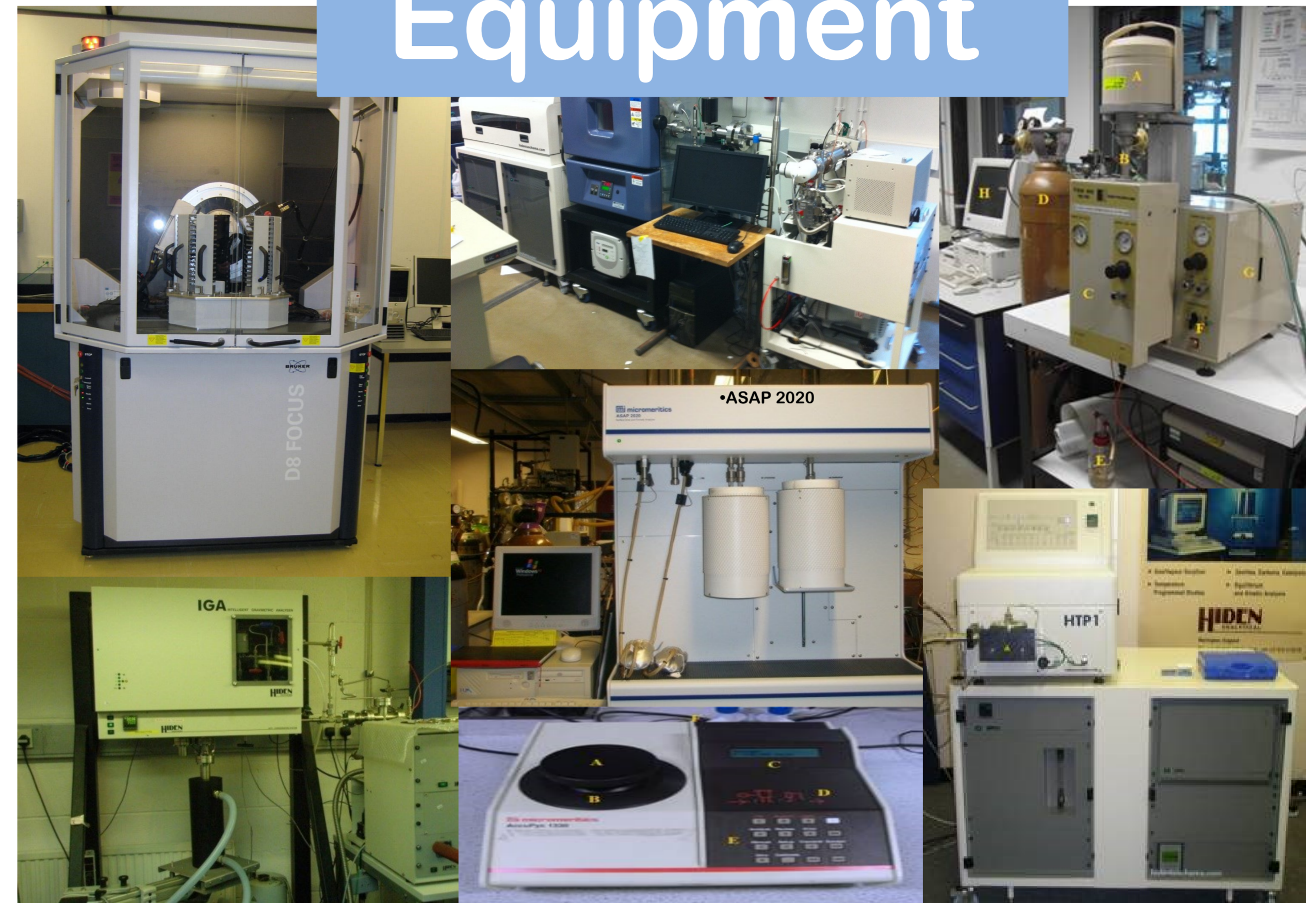
Clockwise from top left: X-ray diffractometer; IsoEx apparatus, Thermal Gravimetric analyser, HTP-1 volumetric sorption analyser, ASAP 2020 sorption analyser (centre), Helium pycnometer and IGA gravimetric sorption analyser
