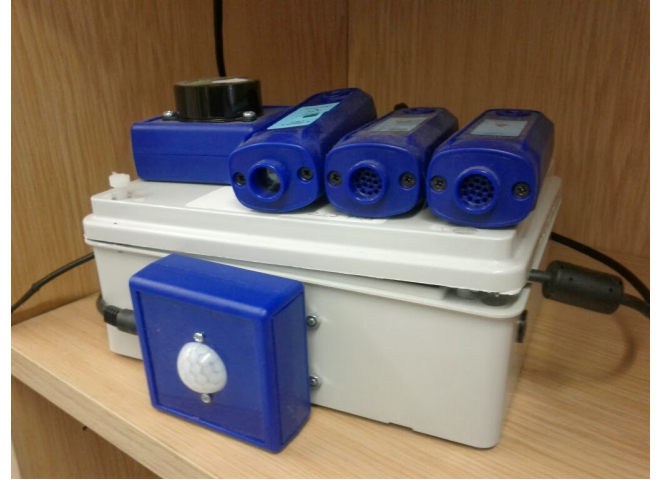
Figure 1: Sensor box in situ. , showing PIR, temperature, CO 2 , light, sound and humidity sensors.
