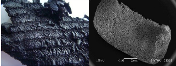
Fig. 1.2. Surface from dry machined rubber and a fully formed chip from cryogenically machined neoprene.
