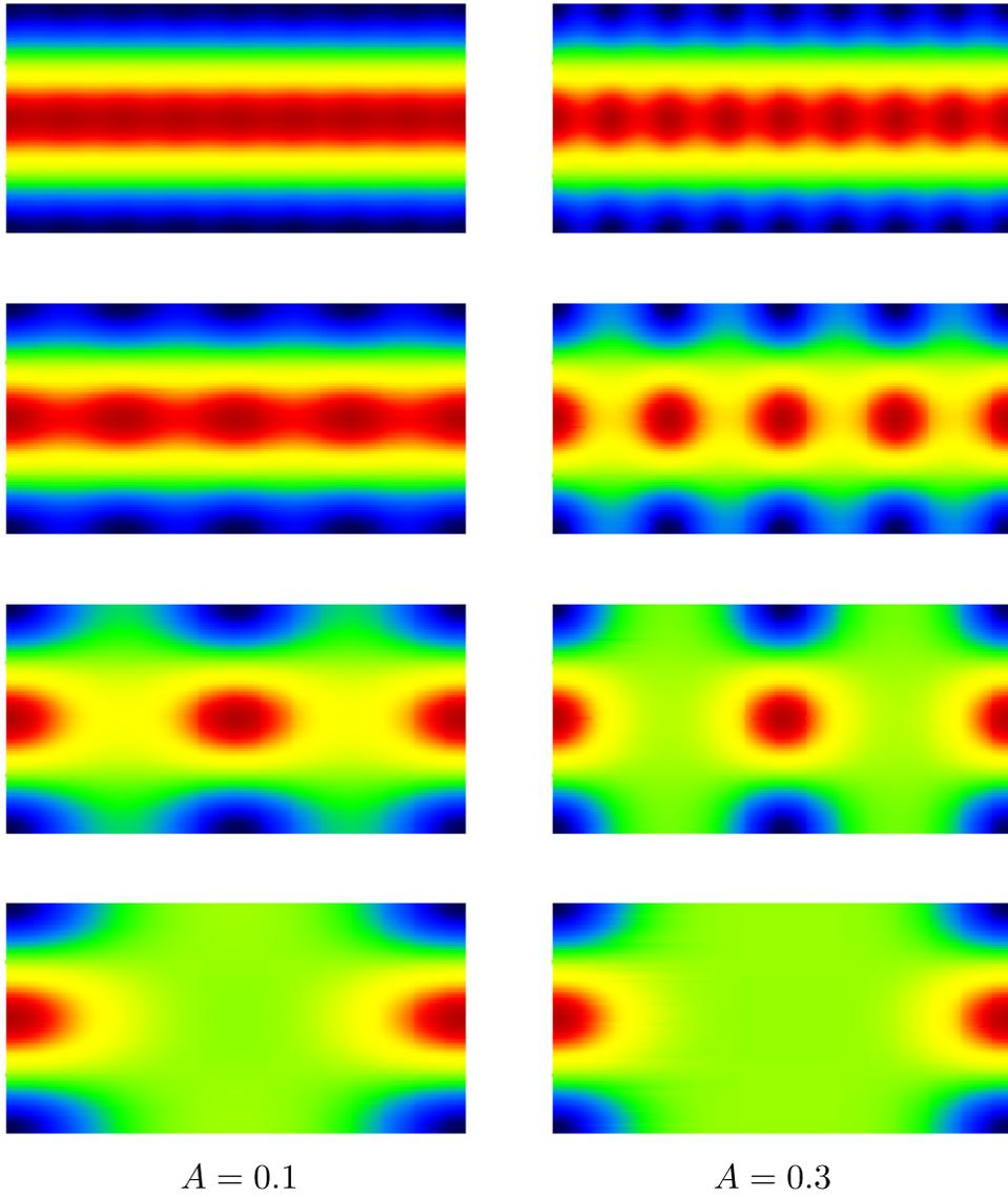
Figure 2: Showing the lower surface rate of heat transfer for different onset modes for  $A = 0.1$  (left) and  $A = 0.3$  (right), and for  $P = 0.5$  (uppermost), 1, 2 and 4 (lowest). Here  $k = \pi$  and  $\nu = 0$  and the shown patterns are confined to  $0 \leq x \leq 4$  and  $0 \leq y \leq 2$ .
