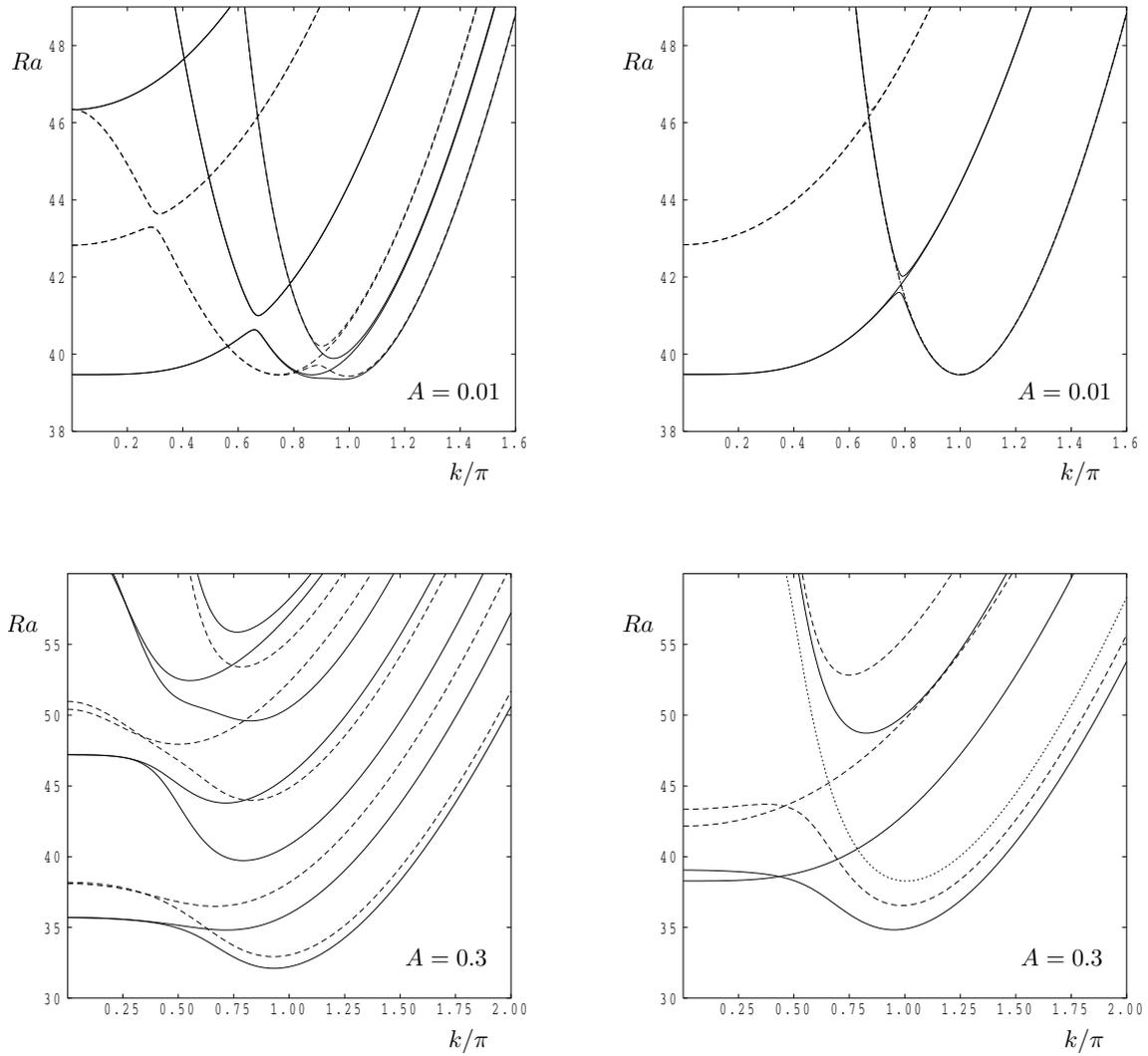
Figure 4: Showing how neutral curves vary with  $P$  for  $A = 0.1$  and  $A = 0.3$ . Here  $k = \pi$  and  $\nu = 0$ . In the two left hand frames continuous lines depict  $P = 4$  and dashed lines  $P = 3$ . In the right hand frames continuous lines depict  $P = 2$ , dashed lines  $P = 1.5$  and dotted lines  $P = 1$ . Up to six modes are displayed.
