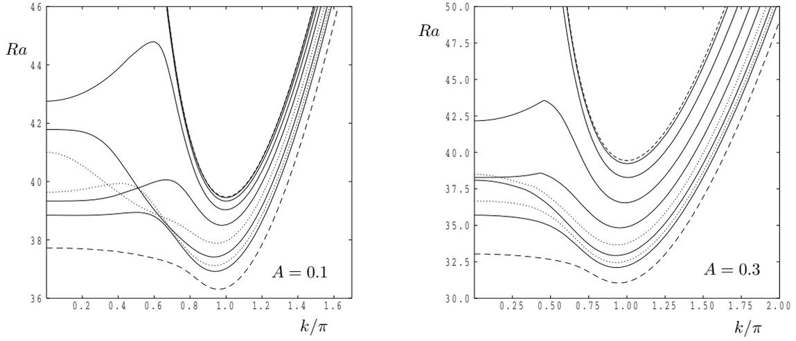
Figure 5: Showing the neutral curves corresponding to the first mode for  $P = 0.2$  (short dashes),  $0.5$ ,  $1$ ,  $1.5$ ,  $2$ ,  $2.5$ ,  $3$ ,  $3.5$ ,  $4$  and  $8$  (long dashes). Curves corresponding to  $P = 2.5$  and  $3.5$  are dotted. Here  $A = 0.1$  (left frame) and  $A = 0.3$  (right frame) with  $k = \pi$  and  $\nu = 0$ .
