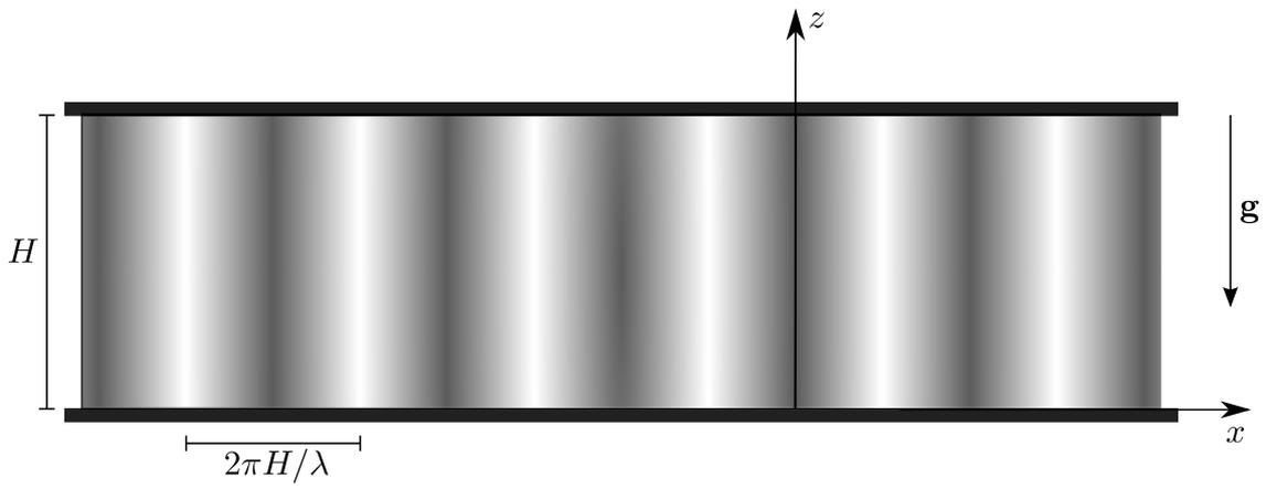
Figure 1: The fluid-saturated porous layer with a periodic horizontal permeability field.
