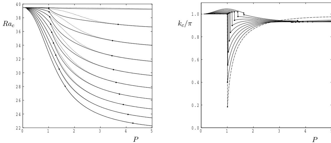
Figure 8: Showing the variation of the critical values of  $Ra_c$  (left) and  $k_c$  (right) with  $P$  for  $A = 0.01, 0.1, 0.2, 0.3 (0.1) 0.9$ . For each  $Ra_c$  curve the two filled circles delineate the range of  $P$  over which  $\nu = 1$  yields the smallest value of  $Ra_c$ , while  $\nu = 0$  elsewhere. For  $Ra_c$  the uppermost line corresponds to  $A = 0.01$ ; for  $k_c$  it is the dashed line.
