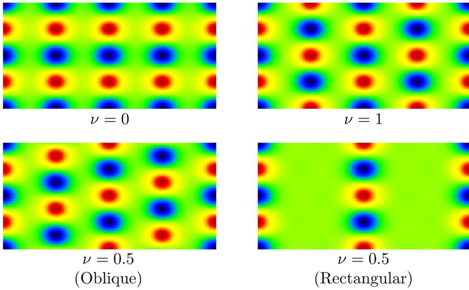
Figure 3: Showing the lower surface rate of heat transfer for different onset modes for the case,  $P = 2$ ,  $A = 0.3$  and  $k = \pi$ , and for the values of  $\nu$  shown.
