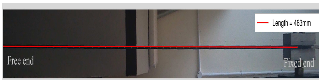
Figure 5. Picture of the cantilever beam setup, fixed end is attached to a mechanical shaker
