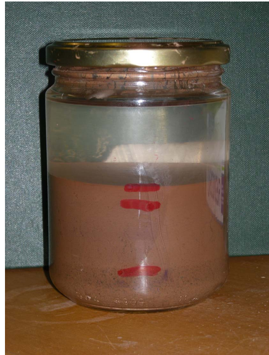
Figure 2. Jar test to determine particle size distribution
