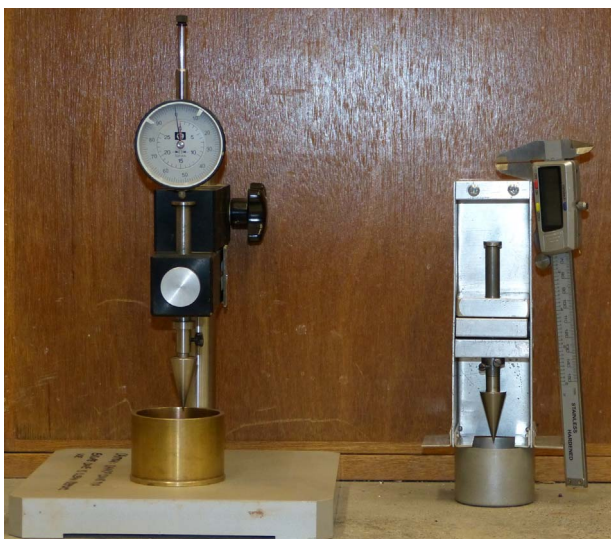
Figure 6. Liquid limit apparatus: commercially available version (left-hand side) and field version (right-hand side)
