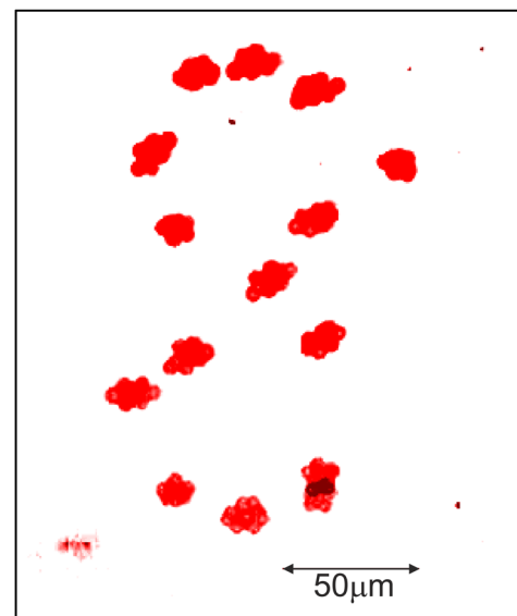
FIG. 4. Manipulation of an agglomerate of 10\ \mu\text{m} polystyrene microspheres in a figure of eight. 14 separate photographs were summed to create this composite view. The contrast was adjusted and a false red colour added to aid viewing.
