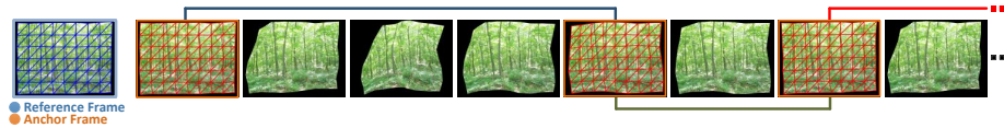
Fig. 2. Step Two. The frames are detected as anchor frames (Red) because of the similar appearance to the reference (Blue). These anchor frames partition the entire sequence into several independent clips which allows tracking performing in parallel.
