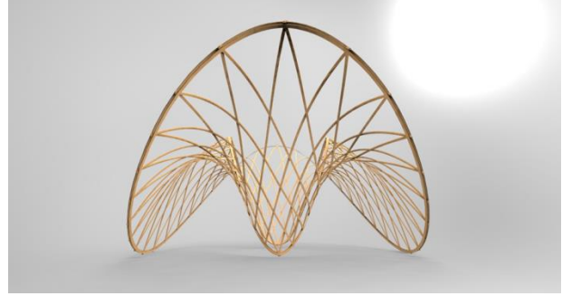
Figure 8: (a) Solar shade that derives its shape from a doubly curved membrane pre-stressed against a three dimensional curved flexible element (PU student project image courtesy S Bagrianski, A Heid, M Krupka) (b) The initial shape of a strained grid shell accounts for straining due to bending and torsion. (SG gridshell image courtesy A Kudless, M Cabrinha and D Shook).
