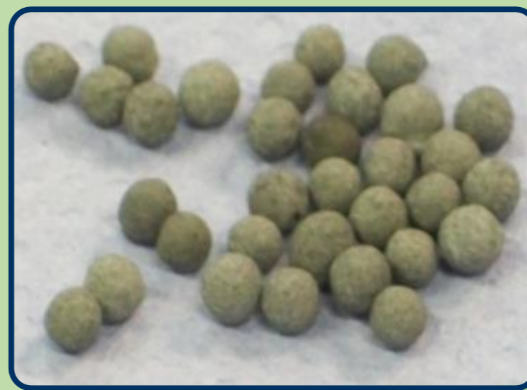
Figure 2 – 1 wt% Pd/Al 2 O 3 pellets
