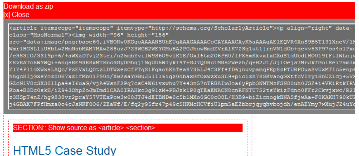
Figure 4. Show5 encodes image data in dataURIs to entire Web pages which can be copied and pasted, for example into a CML (corporate multi-lingual) such as WordPress.
