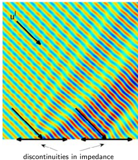
Figure 3.2. Scattered field u^S = u - u^I ; the arrows represent the incident rays, and those diffracted rays scattered at the discontinuities in the impedance which travel in either direction along the boundary.
