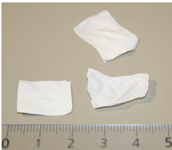
Fig. 7. Electrospun mats peeled from the aluminium foil. The three layered matrix, PCL/PEVA/PCL (left), the two layered matrix with PCL face up (right lower) and PEVA face up (right upper).
