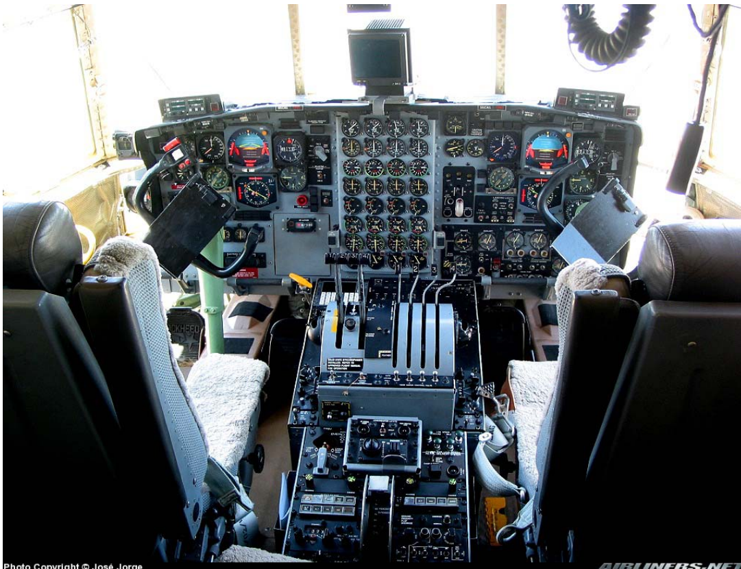
Figure 4.1: Hercules C130-H cockpit layout (printed with permission from José Jorge).
