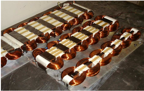
Fig. 4. Experimental concentrated winding linear machines of varying core width, with identical end turn dimensions.
