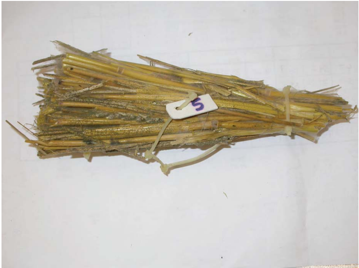
Figure 6: Specimen kept at 98%RH showing volume expansion and mould growth.
