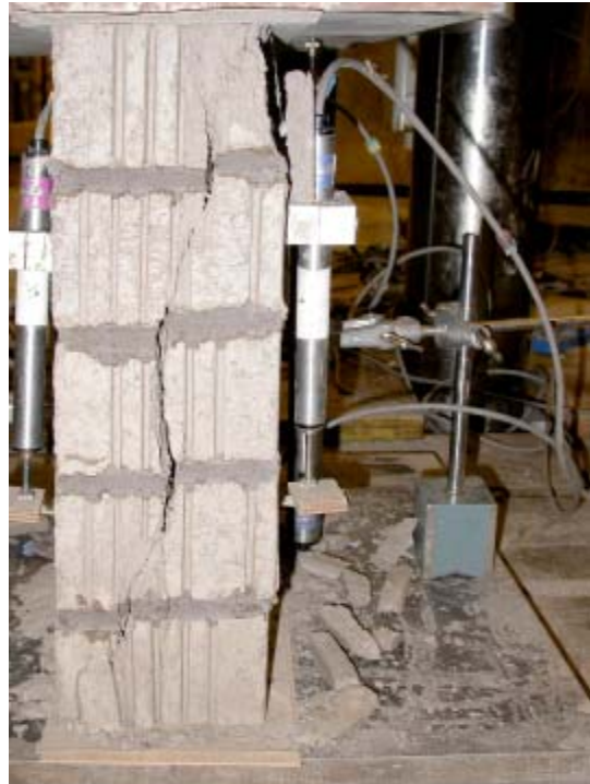
Figure 4: Typical mode of failure for compressive tests
