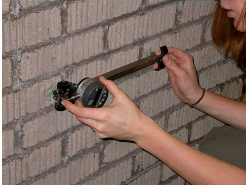
Figure 5: Test wall being measured for dimensional changes
