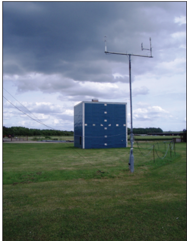
Figure 2. The 6 m Silsoe cube with Airscoop (background), and mast-mounted reference anemometer, directional pitot tube, and static pressure probe (foreground)
