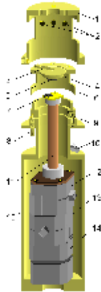
Fig. 2 (colour online) Sketch of a scanning Hall probe microscope head designed to fit on the cold flange of a commercial He-3 refrigerator. 1) receptacle tube, 2) LED array, 3) Bronze flat spring, 4) Sample holder disc, 5) Sample, 6) Sample holder cup, 7) Hall probe, 8) Alignment screw, 9) Extension bronze spring, 10) Electrical connectors, 11) Piezoscanner tube, 12),13) ANPx100 positioners, 14) ANPz100 positioner, 15) Brass microscope hull.
