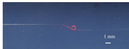
Fig. 4. (Color online) MKR with fiber diameter 4\mu\text{m} and resonator diameter 1 mm embedded in hydrophobic aerogel. The MKR carries red laser light from left to right.
