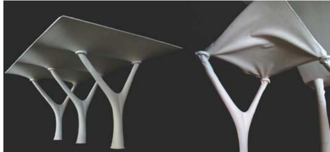
Figure 19 - Fabric cast columns supporting fabric formed shells (image courtesy CAST)
