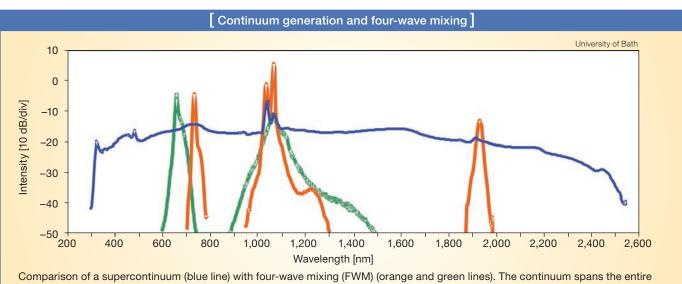
UV-visible-NIR with a smooth spectrum and a relatively low spectral power density. FWM in two different photonic crystal fibers generates high-power density at specific wavelengths for applications such as STED microscopy.
