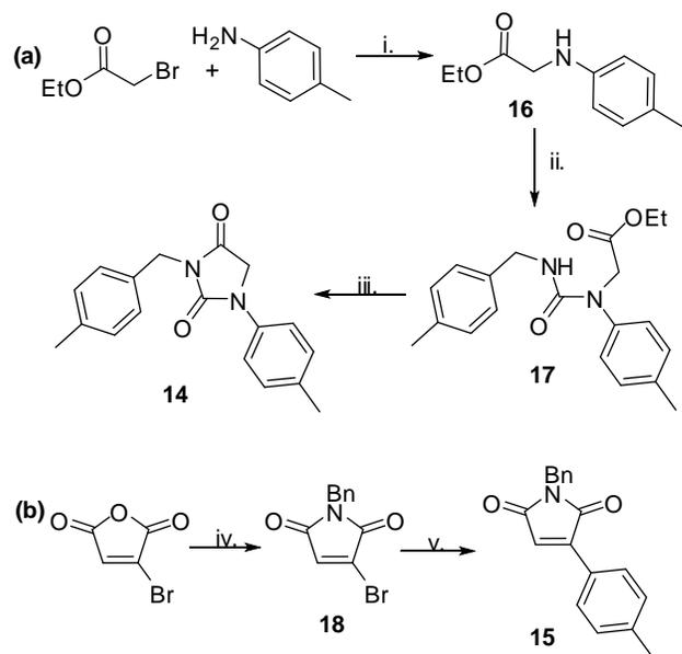
Conditions: i. NaOAc, EtOH, 80 °C, 1 h ii. methyl benzyl isocyanate, toluene, reflux, 5 h iii. NaH, THF, 0 °C - rt, 18 h iv. benzylamine, AcOH, 50 °C, 18 h v. *p*-tolylboronic acid, CsF,  $\text{Cl}_2\text{Pd}(\text{dppf})\cdot\text{CH}_2\text{Cl}_2$ , dioxane, 40 °C, 1 h
