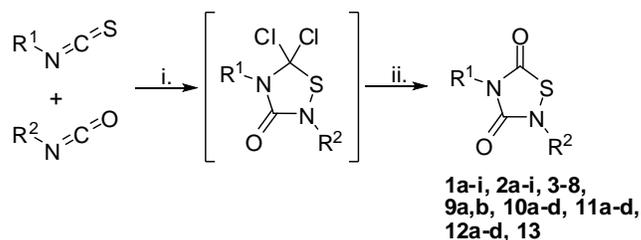
Conditions: i.  $\text{SO}_2\text{Cl}_2$ , THF, 0 °C - rt, 18 h ii. air, 30 min
