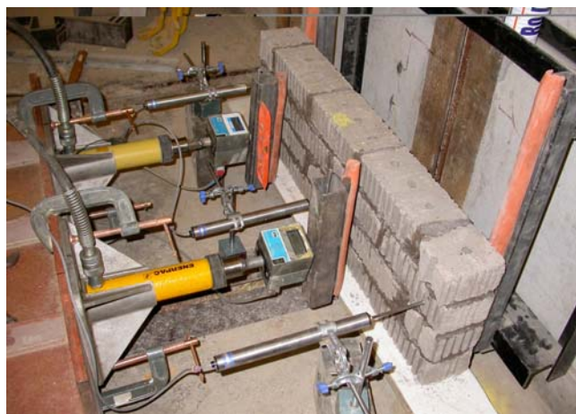
Figure 8. Set-up for flexural tests (perpendicular to bed joint) according to BS EN 1052-2:1999 (BSI, 1999b)
