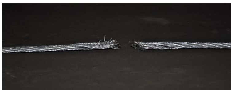
(a) The broken rope defect of the steel cord conveyor belt
