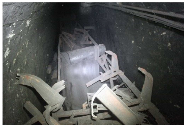
Figure 2. A photo of the steel cord conveyor belt after a fracture failure.
