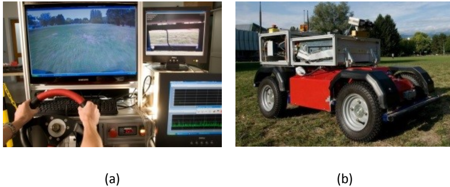
Fig. 7 Drive by Wireless – (a) Driver at remote station using stereo vision (b) Teleoperation test bench Vehicle
