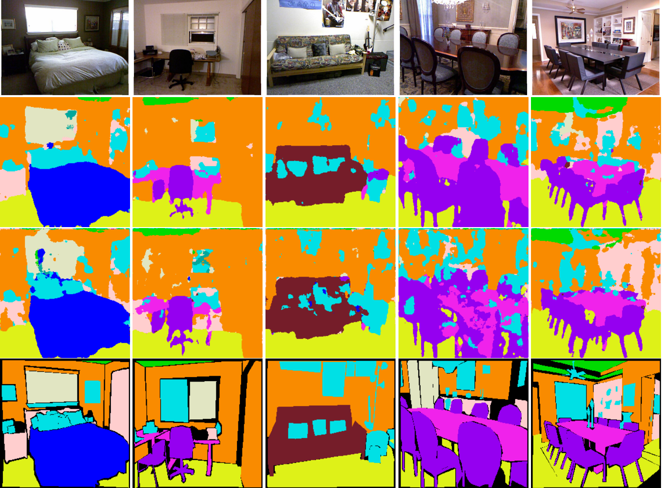
Figure 7. Results for 11 classes on NYUv2 test data obtained with SceneNet-FT-NYU-DHA and NYU-DHA. First row shows the RGB images, predictions returned by SceneNet-FT-NYU-DHA and NYU-DHA are shown in second and third row respectively. Last row shows the ground truth.
