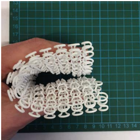
Figure 12. Interlock structure top view.
