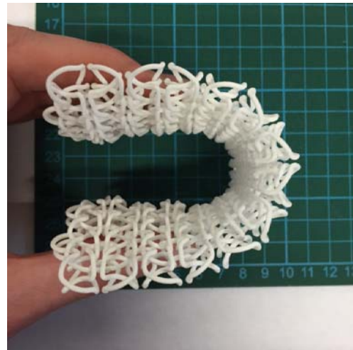
Figure 13. Interlock structure bottom view.
