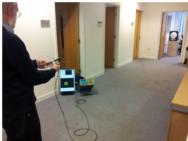
Figure 6. Tethered PU used to measure the radiation pattern of a known radiation source
