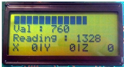
Figure 2. Primary Unit display showing the current measurement value, reading number and spatial position
