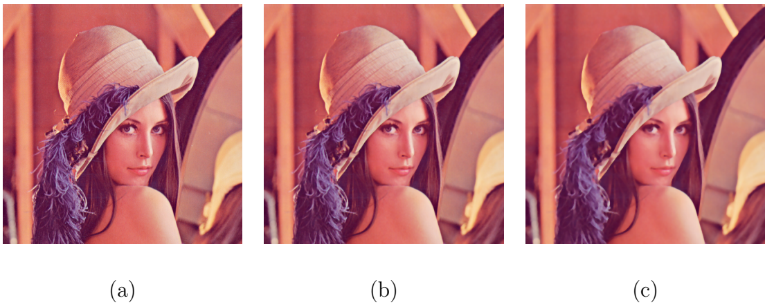
Figure 3.9: (a) Original image; (b) Output image of median filter with 3x3 kernel; (c) Output image of median filter with 5x5 kernel
