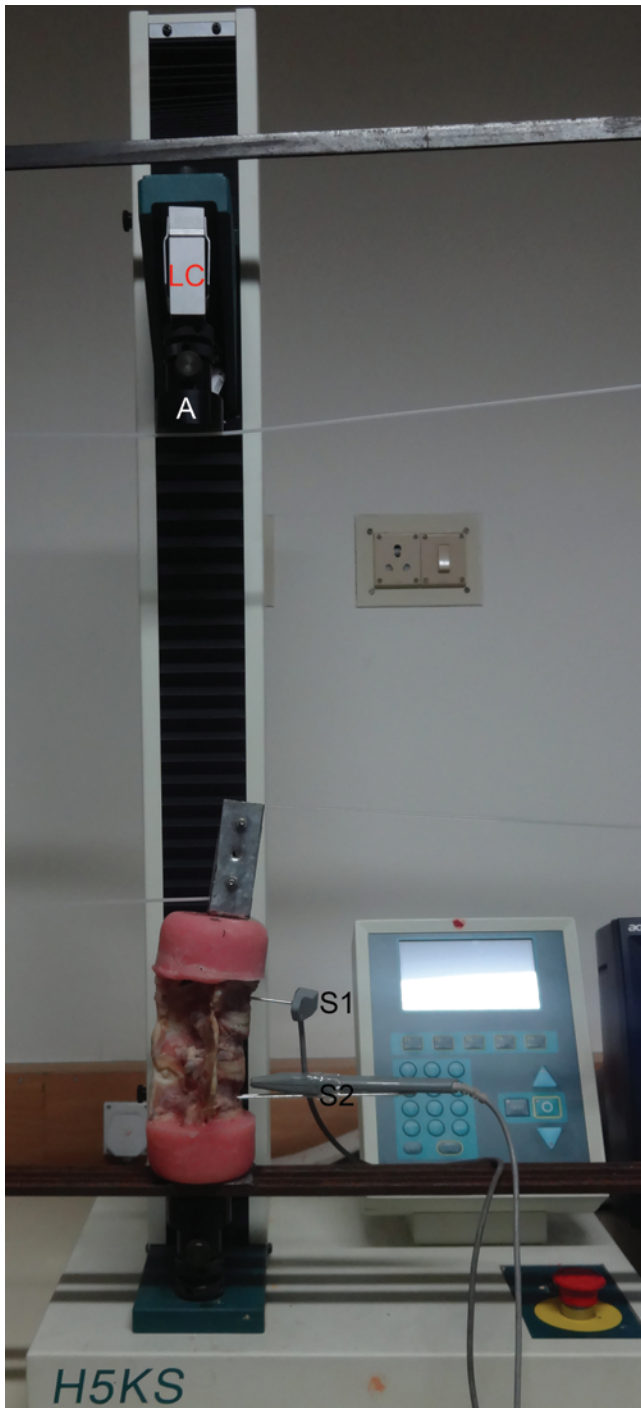
FIG. 4. The test setup for flexion moment. A = actuator; LC = load cell; S1 and S2 = 6-d.f. motion sensors. Figure is available in color online only.
