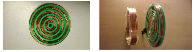
(a) Transmitter coil structure design contains a multiple coils in same plane. (b) Transmitter and receiver coil as used in measurement set-up.
