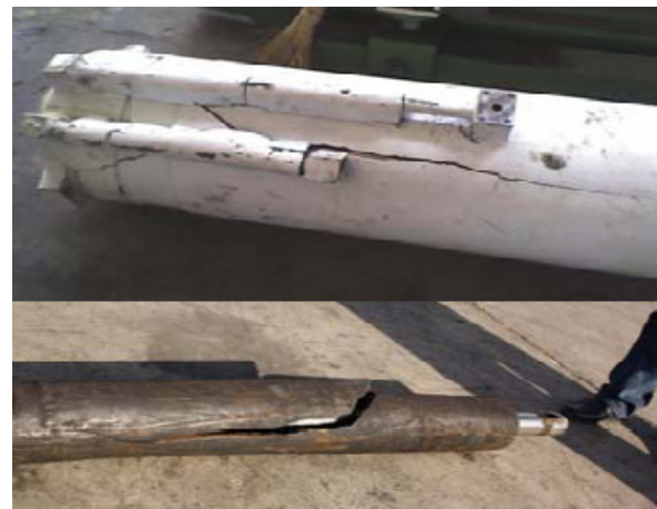
Fig. 1. The damaged hydraulic cylinders
