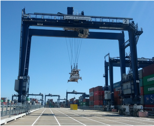
Fig. 1. An RTG crane at the Port of Felixstowe [5].
