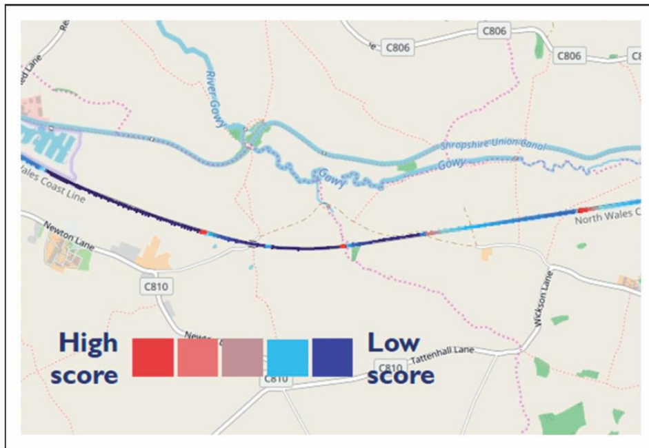
Figure 5. A geographic representation of the data, viewed with the route of the locomotive plotted over an OpenStreetMap geographic map. The line representing the route is coloured to show the relative scoring of each STFT frame. The train is heading north-west.
