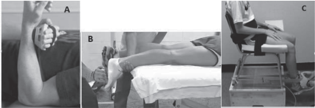
Figure 1. Subject position for A) Elbow flexor muscle strength testing, B) Knee extensor muscle strength testing and C) Ankle plantar flexor muscle strength testing.
