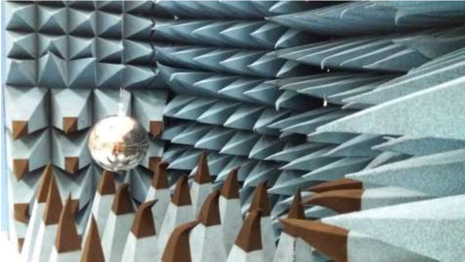
Figure 7. The 86 mm diameter stainless steel sphere suspended on a thin thread of nylon
